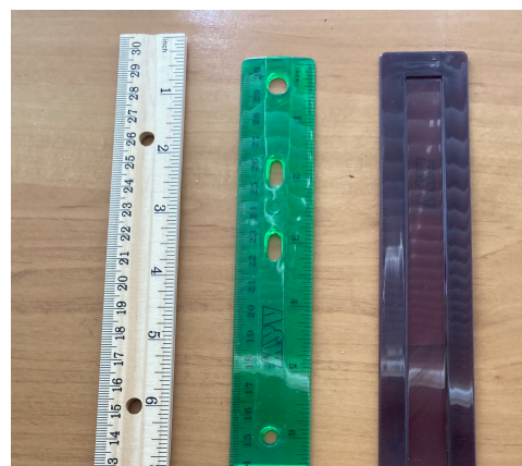
The standard wooden ruler at left is fine; the light-colored plastic ruler is fine—you can see the tic marks and use it. However, the dark-colored ruler on the right is not usable; you cannot see the marks in any normal lighting situation.
