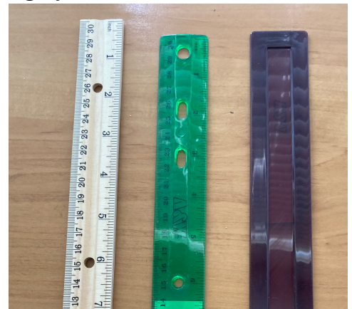
The standard wooden ruler at left is fine; the light-colored plastic ruler is fine—you can see the tic marks and use it. However, the dark-colored ruler on the right is not usable; you cannot see the marks in any normal lighting situation.
